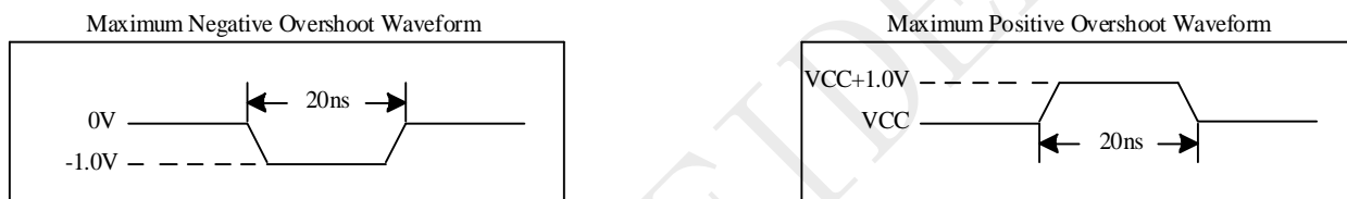
Figure 5-2 Input Test Waveforms and Measurement Level
